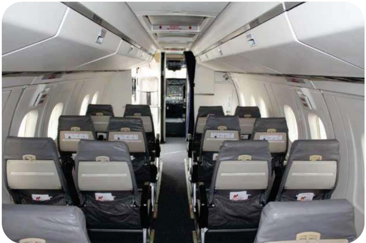
R1 Airlines' *Dash 8-103* has been reconfigured and re-pitched with only 20 passenger seats. The aft bulkhead has also been moved forward for extra cargo/baggage space. R1 refers to it as "The ultimate B1900D replacement," saying that "It can go places and carry loads the 1900 can only dream about." ▶
